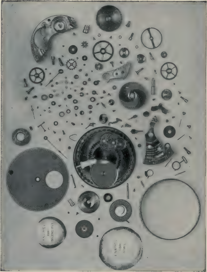
PARTS OF ONE 16 SIZE WALTHAM WATCH MOVEMENT — ACTUAL SIZE. (Illustration used by courtesy of Waltham Watch Company.)
